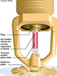
This liquid is designed to expand and break the tube at a certain temperature. The most common are designed to break at 155 degrees. In the average sized room, a 5mm diameter ampule will usually break in about one to one and a half minutes from contact with a heat source. Ampules as thin as 1mm are manufactured for a faster response time.
